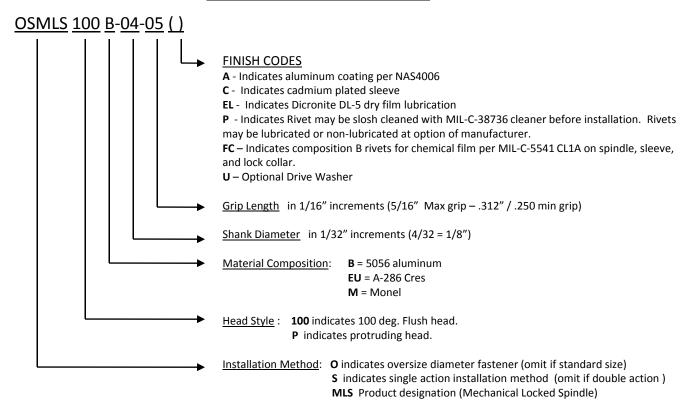
UNIMATIC® Blind Rivets also meet NAS1900 procurement specifications and can be ordered as follows:
